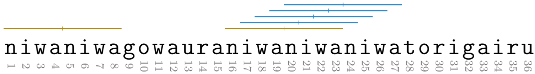
Fig. 3.17: Squares constructed by right rotations. This example highlights all squares of length eight with lines, where the arms of each square are separated with a small vertical bar. Squares that cannot be constructed by right-rotating are colored in dark yellow (■). The other squares are colored in blue (■). These squares can be constructed by right-rotating the square (16, 8).
