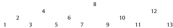
Fig. 4. Geometric interpretation of the 2-fattest numbers. Based on the number line of natural numbers, we move each natural number as many position upwards as it has trailing zeros in its binary representation. In this example of numbers from 1 to 13, the highest number is 8. Now the 2-fattest number of a query interval is the highest number within this range.
