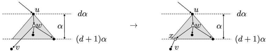
Fig. 2. Splitting the edge (w, v) protruding the boundary of the micro trie rooted at node u by introducing an artificial micro trie node x . The string depth of u is d\alpha while v with a string depth larger than (d + 1)\alpha does not belong to u 's micro trie.
